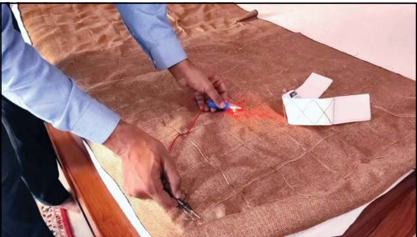
COUNTINUITY TESTING ON ZERO VOLT BEDSHEET
